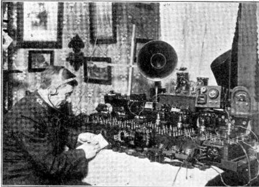
Police Constable William Wooding of the Metropolitan Police Force with his home-made seven-valve set unit and four-valve amplifier on which he has received broadcast telephony from America.
