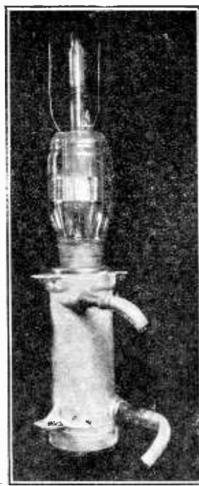
Fig. 109. The valve anode inserted in a water circulated cooling jacket.
